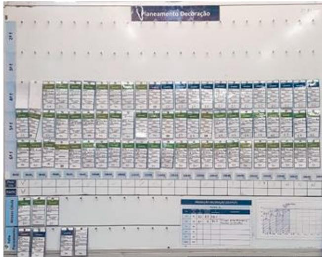
Fig. 4. Production scheduling heijunka box introduced in the decoration process.
