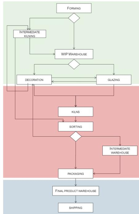
Fig. 1. New products line general process flow.
